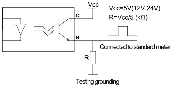
Figure 2 Schematic Diagram of Testing of Electric Energy Pulse
