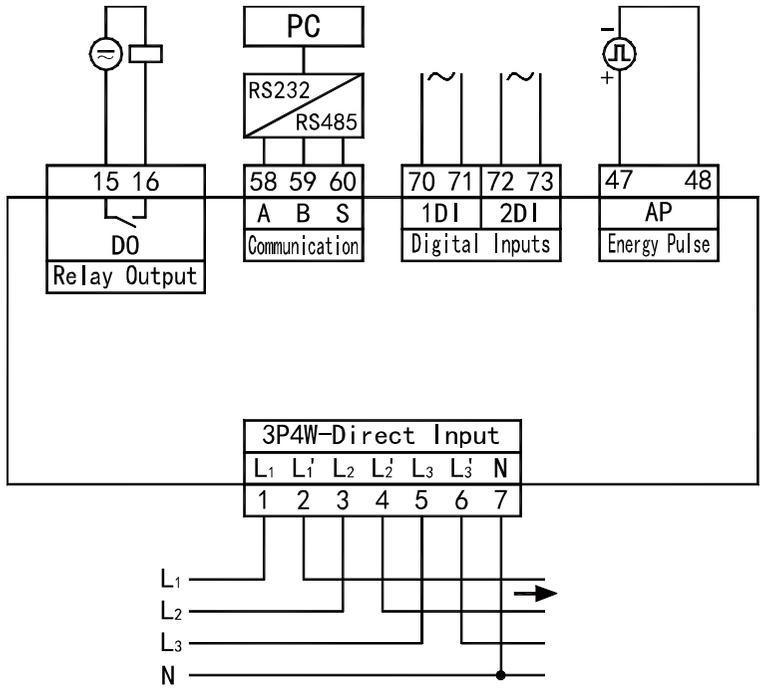
Direct access of three-phase four-wire
