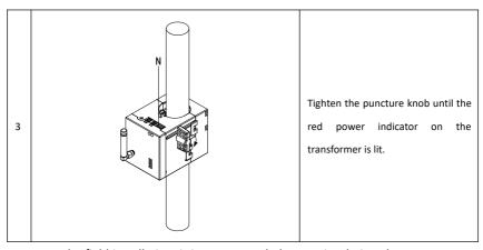
Note: In the field installation, it is recommended to use insulating gloves to operate to prevent electric shock.
